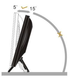
Do not press the LCD screen to change the viewing angle. It may cause damage or break the LCD screen.
